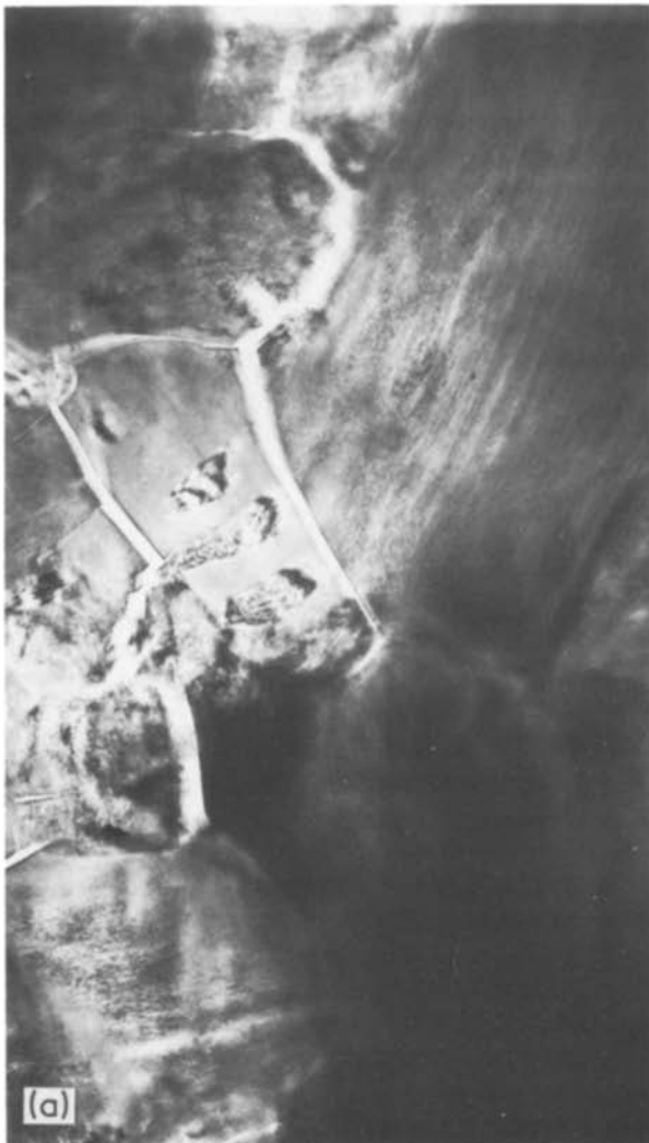
Figure 12 (a) Bright- and (b) dark-field electron microscope images of the general area of the intensely deformed zone beneath the indenter. Note the gross distortion of the faulting within the grains.
